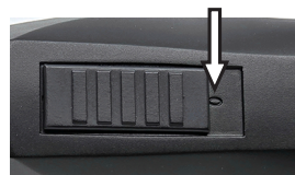
Fig. 4 Switch in OFF-position ("0")
