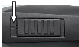
Fig. 5 Switch in ON-position ("I")
